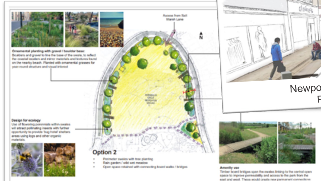
Cornwallis Circle, Whitstable Managing 1.2 hectares of impermeable area with greening; featuring swales and tree planting
